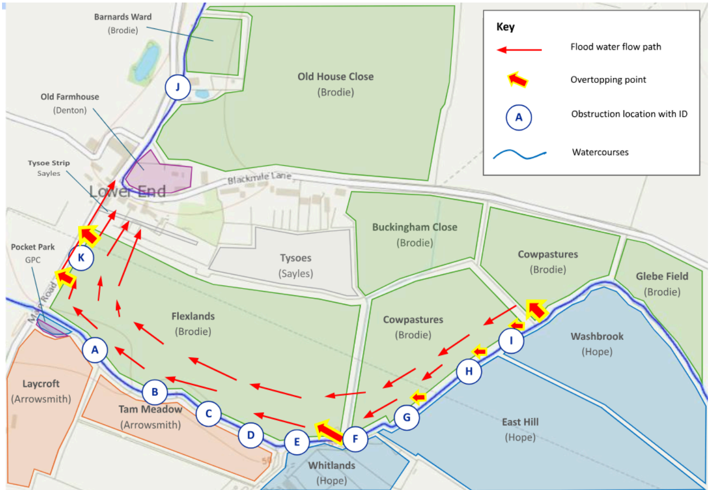
Figure SEQ Figure \* ARABIC 6: Map showing location of obstructions, overtopping points and flow path of floodwater. Map produced with the kind assistance of P. Goffey. © C. Dow
